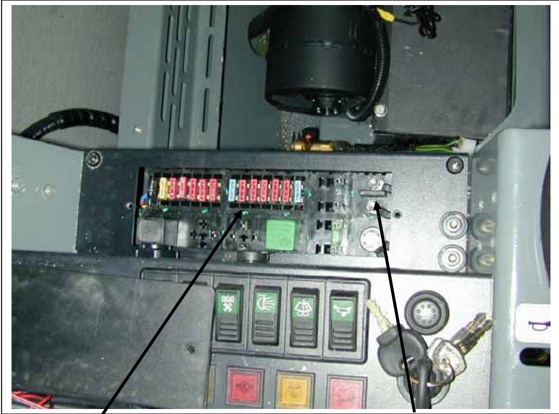
Terminal with ignition live power
